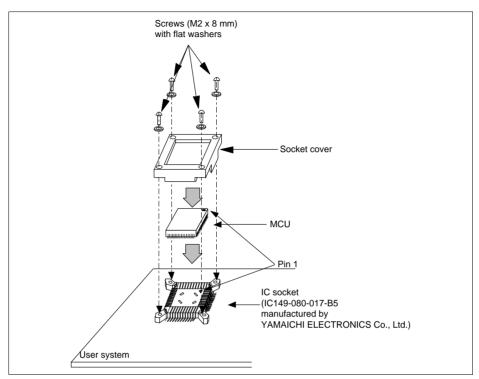
Figure 9 Installing MCU to User System
